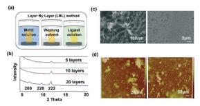
Fig. 1 (a) LBL-D thin film preparation method for the SURMOF. b) Thin film X-ray diffraction analysis of the prepared SURMOF, showing the increasing intensity of the  $2\theta$  value at 11.6 for (222) as the major face. (c) and (d) The SURMOF thin film surface was monitored by SEM and AFM, respectively, to confirm the particle size (nm scale) and the height. The SEM image showed the nanoporous surface of the MOF.
