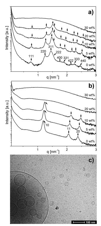
Fig. 1 Composition-dependent SAXS curves of emulsified OA and binary OA/LL-37 mixtures at LL-37 loading varying from 5–30 wt% in OA at (a) pH 7.0 and (b) pH 7.5. Emulsions were stabilized by F127. The identifiable Bragg peaks and further calculated theoretical peak positions are indexed with the corresponding Miller indices. (c) The cryo-TEM image of the OA/LL-37 dispersion containing 30 wt% LL-37 in OA that was prepared at pH 7.5.
