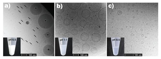
Fig. 3 Representative cryo-TEM images for the emulsions containing 10 wt% LL-37 relative to OA at pH = 6.5 (a), 7.7 (b), and 8.5 (c). The corresponding SAXS curves are presented in Fig. 2. In panel (a), the arrows point towards the smaller self-assemblies, coexisting with the larger EMEs (marked with asterisk). The pictures of the vials show that the dispersions became less turbid with increasing pH from 6.5 (mainly large EME droplets) to 8.5 (mainly small vesicles and micelles).
