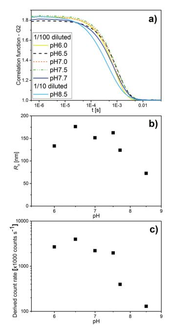
Fig. 4 (a) pH-Dependent DLS correlation functions for emulsions containing 10 wt% LL-37 in OA at different pH values in the range of 6.0-8.5. (b) The corresponding  $R_{\rm H}$  values determined with the cumulative analysis from the correlation functions in (a) (see also Table SI2† for the corresponding  $R_{\rm H}$  and PDI values). (c) The corresponding light scattering intensity in this pH range.
