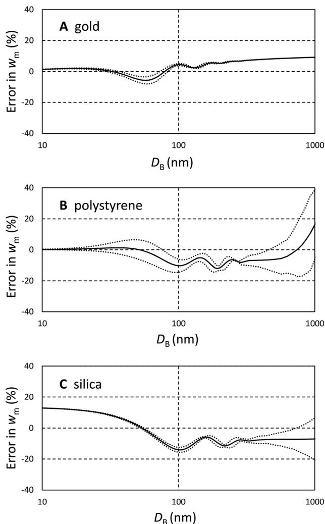
Fig. 2 Error in measured relative dimer to primary mass concentration,  $w_m$  for three typical materials. The bias due to shape effects is shown as solid lines and the estimated errors due to incorrect size and refractive index are shown as dotted lines indicating ranges either side of the bias. (A) Gold. (B) Polystyrene. (C) Silica.
