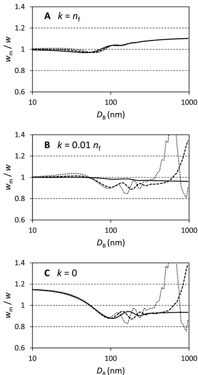
Fig. 1 Ratio of the measured dimer to primary particle relative mass concentration to the true value in DCS for spherical primary particles as a function of primary particle diameter  $D_B$ . Solid lines are for particles with  $n = 1.41$ , dashed lines  $n = 1.68$ , and dotted lines  $n = 1.94$ . (A) Materials which strongly absorb light. (B) Materials which weakly absorb light. (C) Transparent materials.
