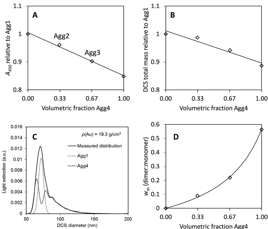
Fig. 4 Results from agglomerated samples. (A) UV-vis absorbance at 450 nm,  $A_{450}$ , normalised to the monomodal sample, Agg1. (B) Total mass of particles from DCS normalised to the monomodal sample, Agg1. (C) Fit to DCS data for sample Agg3, using descriptions of Agg1 and Agg4 data. (D) Relative mass of dimers to monomers from DCS,  $w_m$ . Lines are fits to the data, in (A) and (B) they are linear, for D eqn (7) is used with  $a = 3.1$ .
