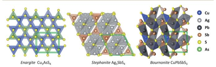
Fig. 2 Illustrations of the crystal structures of candidate solar minerals: enargite (space group  $Pmn2_1$ ), stephanite (space group  $Cmc2_1$ ), and bournonite (space group  $Pmn2_1$ ).
