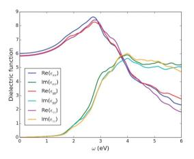
Fig. 10 Three components of the calculated dielectric function,  $\varepsilon(\omega)$ , as a function of incident photon energy,  $\omega$ , for stephanite (Ag<sub>5</sub>SbS<sub>4</sub>).
