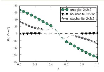
Fig. 14 Spontaneous polarisation along a path connecting the structures with  $+P_s$  and  $-P_s$  for enargite (Cu<sub>3</sub>AsS<sub>4</sub>), stephanite (Ag<sub>5</sub>SbS<sub>4</sub>) and bournonite (CuPbSbS<sub>3</sub>). The markers indicate points calculated with 2 × 2 × 2 k-points and the dashed line is the path obtained using 1 × 1 × 1 k-points. The curves are set to pass through 0 for  $\lambda = 0.5$ . See ESI† for further details.
