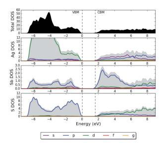
Fig. 9 HSE06 + SOC partial electronic density of states (pDOS) of stephanite ( $Ag_5SbS_4$ ), where the top of the valence band has been set to 0 eV
