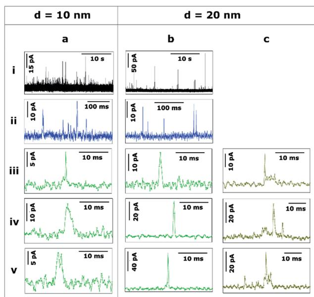
Fig. 3 Representative current transients obtained by applying  $E = +0.6$  V vs. Ag/AgCl to a GC electrode with a solution containing Ag NPs with nominal diameter of (a) 10 nm and (b and c) 20 nm. The numbers i–v refer to different cases discussed in the text.
