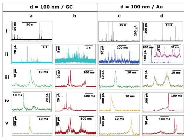
Fig. 5 Representative current transients obtained by applying  $E = +0.6$  V vs. Ag/AgCl to a (a and b) GC and a (c and d) Au electrode with a solution containing Ag NPs with nominal diameter of 100 nm. The numbers i–v refer to different cases discussed in the text.
