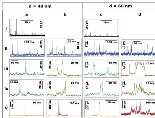
Fig. 4 Representative current transients obtained by applying  $E = +0.6$  V vs. Ag/AgCl to a GC electrode with a solution containing Ag NPs with nominal diameter of (a and b) 40 nm and (c and d) 60 nm. The numbers i–v refer to different cases discussed in the text.
