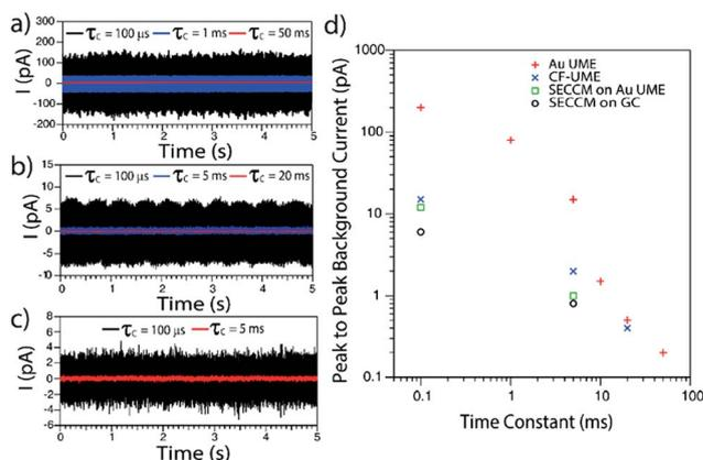
Fig. 2 Representative  $I-t$  transients obtained during the polarization at  $E = +0.6$  V vs. Ag/AgCl of a (a) Au UME, (b) CF-UME and (c) GC electrode in SECCM setup, with different amplification time constants. (d) Peak to peak background current vs. amplification time constant for different electrode materials and setups.
