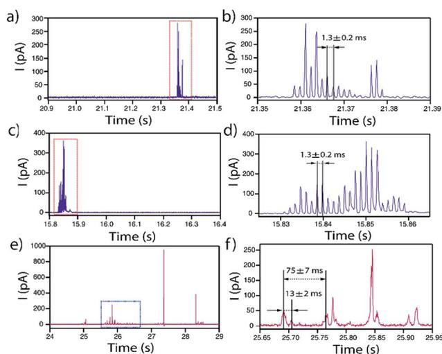
Fig. 10 Representative periodic  $I-t$  transients obtained by applying  $E = +0.6$  V vs. Ag/AgCl to a GC with a solution containing Ag NPs with nominal diameter of (a and b) 40 nm and (c and d) 60 nm, and to Au with a solution containing Ag NPs with nominal diameter of (e and f) 100 nm.
