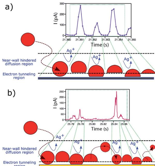
Fig. 11 Periodic  $I-t$  patterns (from Fig. 10) and schematic representation of the electrochemical dissolution mechanism of Ag NPs on a (a) GC and on (b) Au substrate.
