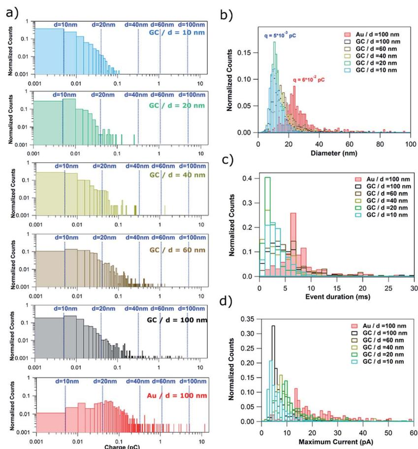
Fig. 6 (a) log-log plot of the charge histograms for single events recorded during the stripping of Ag NPs with nominal diameter of 10, 20, 40, 60 and 100 nm on GC and 100 nm Ag NPs on Au electrodes. Histograms of the (b) equivalent NP diameter (assuming dissolution of whole NP), (c) event duration and (d) maximum current.
