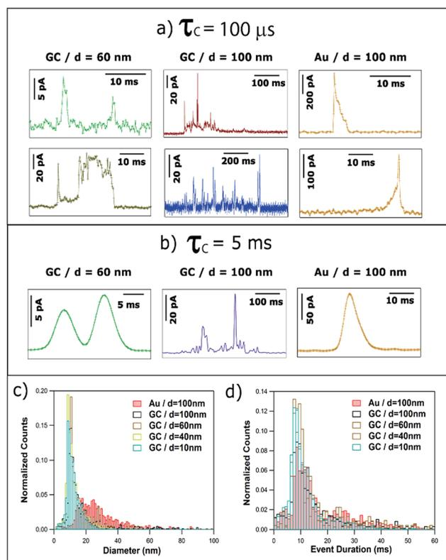
Fig. 8 Representative current transients obtained with (a)  $\tau_C = 100 \mu\text{s}$  and (b)  $\tau_C = 5$  ms, by applying  $E = +0.6$  V vs. Ag/AgCl to a GC electrode with a solution containing Ag NPs with nominal diameter of (left) 40 nm and (middle) 100 nm, and to a Au electrode with a solution containing Ag NPs with nominal diameter of 100 nm (right). Histograms of (c) equivalent NP diameter (assuming complete dissolution of NPs) and (d) event duration, both for  $\tau_C = 5$  ms.
