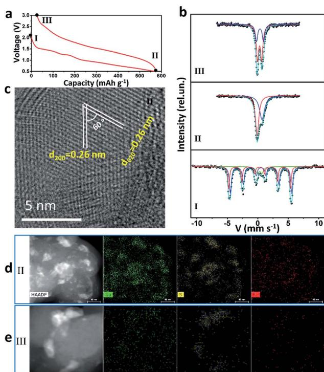
Fig. 3 (a) Discharge–charge curves of the first cycle at the specific current of 0.2 A g<sup>-1</sup>; (b) <sup>57</sup>Fe Mössbauer spectra, (c) TEM image, (d) STEM and (e) EDS mappings of the as-prepared Fe<sub>3</sub>S<sub>4</sub> at different states.
