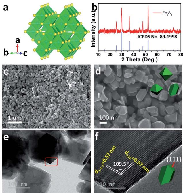
Fig. 1 Structure characterization of the as-prepared  $\text{Fe}_3\text{S}_4$ . (a) Crystal structure and (b) XRD pattern of the as-prepared  $\text{Fe}_3\text{S}_4$ . (c and d) SEM images, (e) TEM and (f) HRTEM images for the as-prepared  $\text{Fe}_3\text{S}_4$ .
