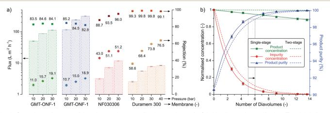
Fig. 6 Separation performance of the solvent-resistant nanofiltration membranes for 2-imidazoline product purification: ■ and ◆ indicates rejections for 1, and the corresponding benzaldehyde substrate impurity, respectively (a). Purification performance for single-stage and two-stage diafiltration processes. Solid and dashed lines represent the simulated performance based on rejections, while symbols signify experimental points to validate the model used for simulation (b).
