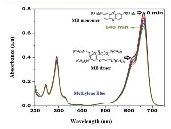
Fig. 7 Time dependent MB absorption spectra for the 0.055 wt% Au-HAp nanocomposite used to determine its photocatalytic activity.
