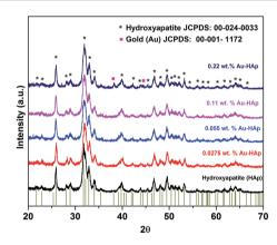
Fig. 2 XRD spectra of HAp and Au-HAp nanocomposites with different Au contents. The bottom vertical bars show the peak positions of pure hydroxyapatite in hexagonal phase (JCPDS: 00-024-0033).
