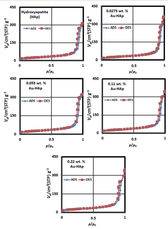
Fig. 4 N<sub>2</sub> adsorption-desorption isotherms of HAp and Au-HAp nanocomposites.
