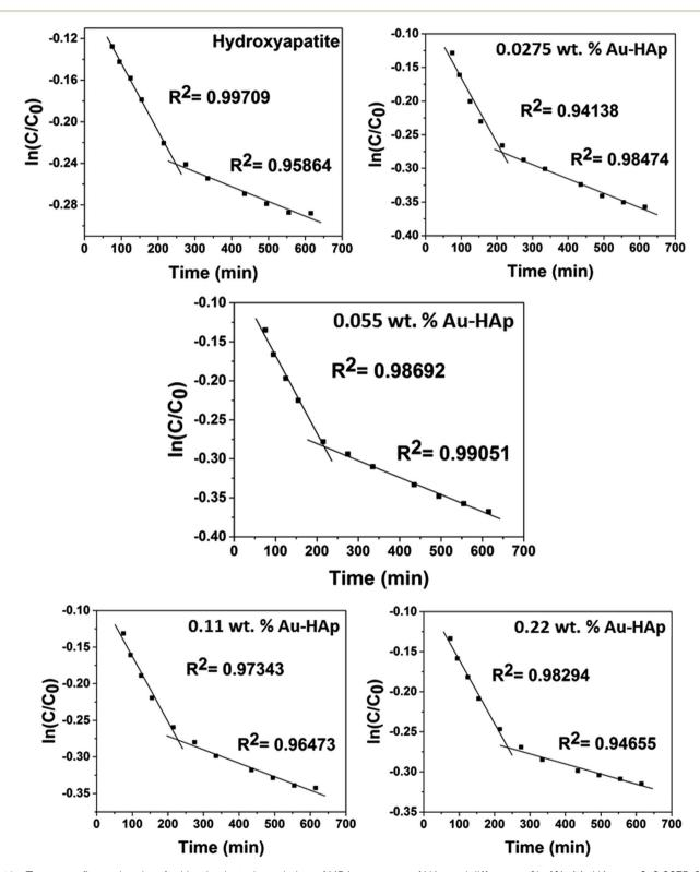
Fig. 10 Two stage first order plots for kinetic photodegradation of MB in presence of HAp and different wt% of [Au(x)-HAp, x=0, 0.0275, 0.055, 0.055]0.11, 0.22 wt%] Au-HAp nanocomposites.
