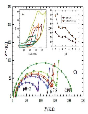
Fig. 5 (A) Cyclic voltammograms of 1.0 mM DAC in B-R buffer at different pH values, with scan rate 100 mV s<sup>-1</sup> recorded at CPE/Cs/ CNT-Co. (B) Graph of current response of DAC at different pH values using bare CPE and CPE/Cs/CNT-Co. (C) Nyquist plots for DAC using bare CPE and CPE/Cs/CNT-Co in B-R buffer with different pH values.
