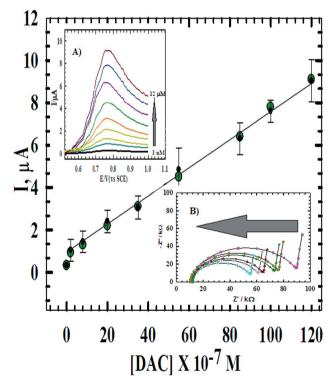
Fig. 8 The calibration curve of DAC at CPE/Cs/CNT-Co. Inset (A) DPV of the successive additions of DAC in B-R buffer and 10 mV s $^{-1}$ . Inset (B) the Nyquist plot of the successive additions of DAC.
