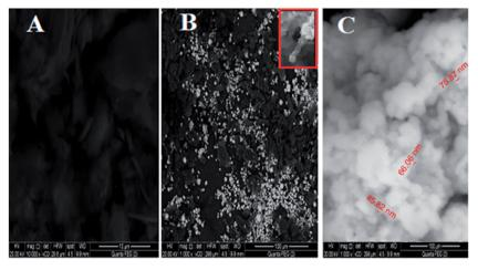
Fig. 2 The SEM of (A) bare CPE, (B) CPE/Cs/CNT and (C) CPE/Cs/CNT-Co
