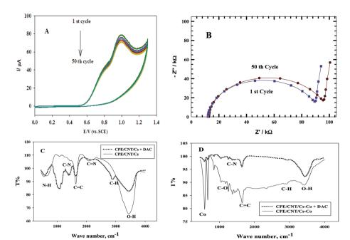
Fig. 10 (A) Repeated CVs of 1 mM DAC in B-R buffer (pH = 2.0) at CPE/Cs/CNT-Co for 50 times. (B) Impedance spectroscopy of the first and the 50<sup>th</sup> cycles of 1 mM DAC in B-R buffer (pH = 2.0) at CPE/Cs/CNT-Co (C) FT-IR spectrum of CPE/Cs/CNT in the presence and absence of DAC (D) FT-IR spectrum of CPE/Cs/CNT-Co in the presence and absence of DAC.
