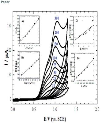
Fig. 6 Cyclic voltammograms (CV) of 1.0 mM DAC at CPE/Cs/CNT-Co in B-R buffer pH 2.0 at: 10, 25, 50, 75, 100, 150, 200 and 300 mV s<sup>-1</sup> Inset (A) plot of the anodic peak current values versus square root of scan rate. Inset (B) plot of log the anodic peak current versus log the scan rate. Inset (C) plot of the anodic peak potential values versus In scan rate. Inset (D) plot of the anodic peak potential values versus scan rate.
