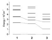
Fig. 4 Energy level diagram of the splitting of the ground <sup>4</sup>F term for a free Co(II) ion in the ligand field of 1, 2 and 3. This diagram was extracted from ab initio spin-free calculations, and each black line corresponds to a spin-free quartet without SOC. The orbital degeneracy is broken down by the actual geometry, resulting in seven quartets for each complex.
