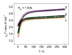
Fig. 2 Temperature dependence of  $\chi_{\rm m}T$  between 2 and 300 K for crystalline powder samples of 1-3 (dots are values obtained in SQUID; lines correspond to ab initio calculations and scaled by 0.92).
