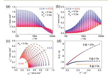
Fig. 3 Frequency dependence of the (a) in-phase ac susceptibility ( $\chi'$ ), and (b) out-of-phase ac susceptibility ( $\chi''$ ) under zero dc field for 3. (c) Cole-Cole plots for 3 under zero dc field. The solid lines indicate fitting using a generalized Debye model. (d) ln  $\tau$  vs.  $T^{-1}$  plots for 3 and 5. The red triangles were collected from SQUID, while the other data were collected from PPMS. The solid blue lines correspond to fitting to the relaxation processes.
