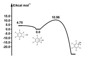
Fig. 1 Schematic energy path for the addition of hydroxyl radicals to hexafluorbenzene. The values obtained by the G3 method are enthalpies at room temperature (298.15 K) relative to the prereaction complex in kcal mol<sup>-1</sup>. Reprinted from ref. 83 with the permission of Croatian Chemical Society according to CC BY license (https://creativecommons.org/licenses/by/4.0/).
