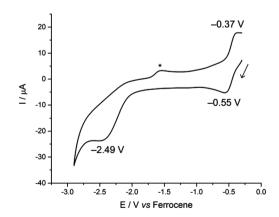
Fig. 3 Cyclic voltammogram of 3, measured at 100 mV s $^{-1}$  in 0.1 M CH<sub>2</sub>Cl<sub>2</sub>/[ $^{n}$ Bu<sub>4</sub>N][BPh<sub>4</sub>]. The asterisk denotes a decomposition product that is formed only after the irreversible reduction.
