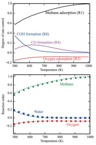
Fig. 1 Top: Numerical values for the degree of rate control in methane oxidation over Pd(100). The simulations are performed with the full model of ref. 3. Bottom: Reaction orders in the methane, water, and oxygen pressure as a function of temperature. The lines are evaluated by eqn (8), and the points are obtained from the total rate of the full microkinetic model. Pressures:  $p_{CH_4}$  = 0.61 mbar,  $p_{O_2}$  = 3.06 mbar, and  $p_{H_2O} = 0.01$  mbar.
