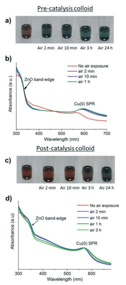
Fig. 6 a & b) Photographs and UV/vis spectra of the pre-catalysis CuMesZnO@DOPA solution before and after air exposure. c & d) Photographs and UV-vis spectra of the CuMesZnO@DOPA postcatalysis solution before and after air exposure.
