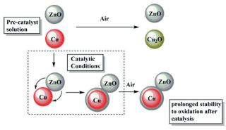
Fig. 7 Schematic illustrating the proposed oxidation of Cu(0) NPs by air before or after catalysis, with the formation of a Zn containing surface layer during catalysis.
