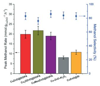
Fig. 2 Peak methanol rates and selectivity for the colloidal CuZn@DOPA catalysts, and the reference CuZnO@St and Cu-ZnO-Al<sub>2</sub>O<sub>3</sub> catalysts in the hydrogenation of CO<sub>2</sub> to methanol. Reaction conditions: 210 °C, 50 bar, H2: CO2 molar ratio of 3:1, 10.8 Lsyngas mmol<sub>Cu+Zn</sub><sup>-1</sup> h<sup>-1</sup> in mesitylene.
