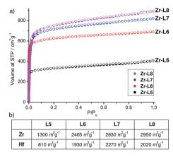
Fig. 6 (a)  $N_2$  adsorption isotherms (77 K) for Zr-L5, Zr-L6, Zr-L7 and Zr-L8. (b) BET surface areas for all Zr and Hf MOFs, as derived from their  $N_2$  adsorption isotherms.
