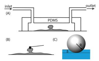
Fig. 1 (A) Experimental set up of the flow cell showing the biofilm growing on the glass surface of the chamber. (B) AFM cantilever with a spherical polystyrene tip of radius 5  $\mu$ m was used to probe the surface of the biofilm. (C) The Young's modulus was measured from the indentation depth for a given force.
