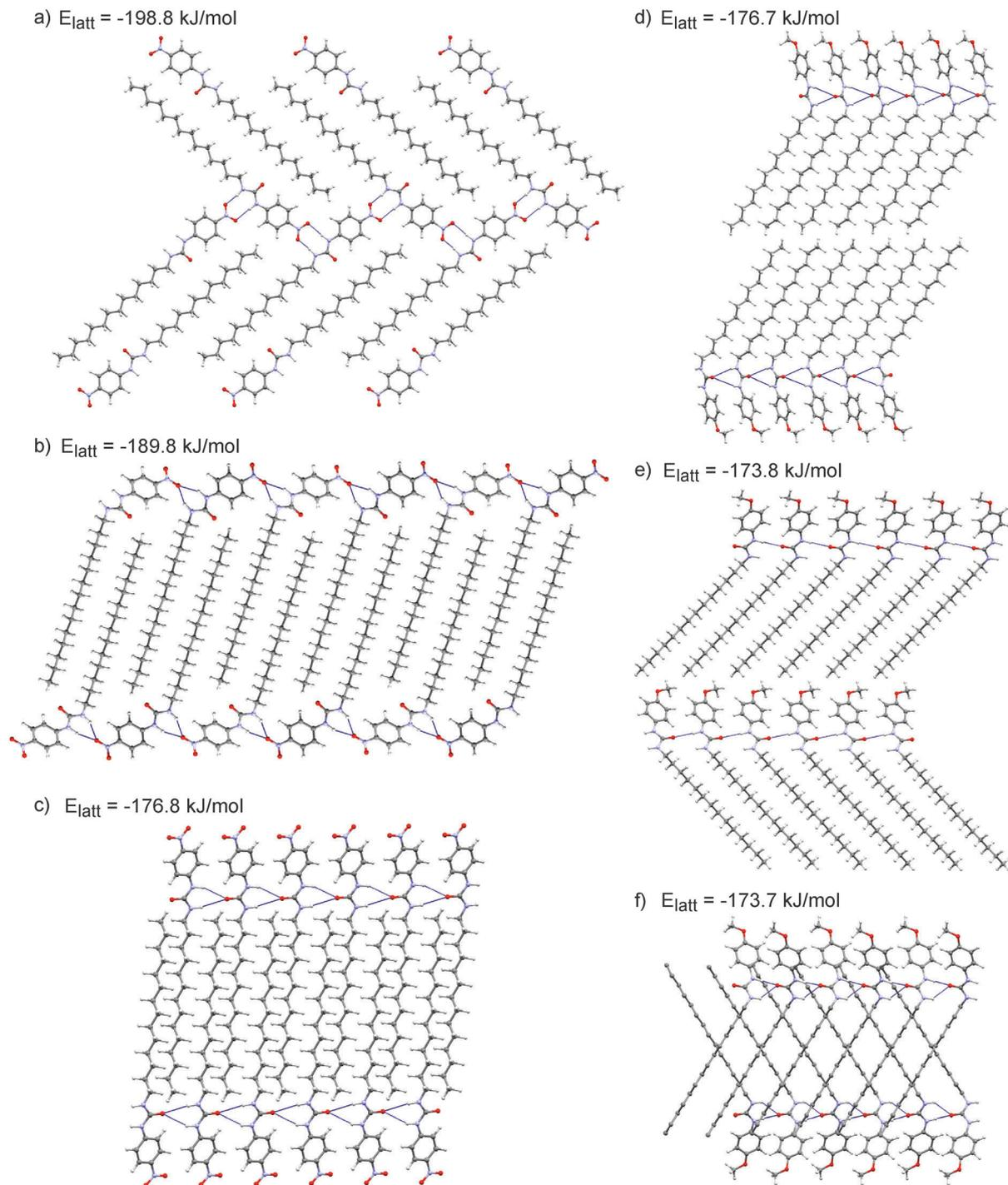
Fig. 4 Molecular packing in representative low energy predicted crystal structures of **14** (a–c) and **15** (d–f). (a and d) Are the global minimum energy crystal structures that have been located for each molecule. Calculated lattice energies of each structure are shown. Hydrogen bonds are shown as dashed blue lines. Hydrogen atoms on the alkyl chains are hidden in (f) for clarity.
