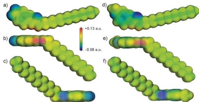
Fig. 3 Calculated molecular electrostatic potentials of **14** (a–c) and **15** (d–f). The potentials are plotted on the 0.02 a.u. electronic isodensity surface. The red patches of positive electrostatic potential in (b) and (e) correspond to the urea hydrogen atom positions. (c and f) Show the view down the urea oxygen atom, highlighting its negative electrostatic potential.
