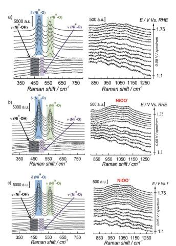
Fig. 2 SER spectra obtained at constant potential during the electrochemical oxidation of Ni(OH)<sub>2</sub> and the subsequent OER on NiOOH at different pH's. The ionic strength of the solution was fixed to 0.1 M with NaClO<sub>4</sub> except for pH 13, that solution is NaOH 0.1 M. The left panel presents the spectra in the wavenumber region  $300-800 \text{ cm}^{-1}$  and the right panel presents the wavenumber region  $800-1300 \text{ cm}^{-1}$ : (a) pH 11, (b) pH 12.0, (c) pH 13.0.
