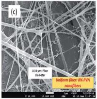
Fig. 8 SEM micrographs of PVA nanofibers indicating the effect of polymer concentration on fiber quality and fiber diameter (a) 4% PVA (b) 6% PVA (c) 8% PVA  $[M_w: 146\ 000-186\ 000, 99+\% hydrolysed, solvent used: deionised water].$
