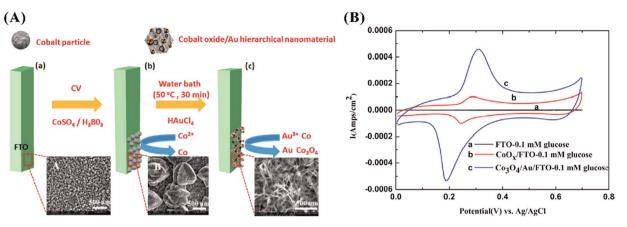
Fig. 5 (A) Shows the fabrication of  $Co_3O_4$ /Au hierarchically nanostructured electrode, and (B) presents cyclic voltammograms of the bare FTO,  $CoO_x$ /FTO, and  $Au/Co_3O_4$ /FTO in 0.1 M NaOH solution with the presence of 0.1 mM glucose. Adapted with permission from ref. 112. Copyright @ 2016 American Chemical Society.
