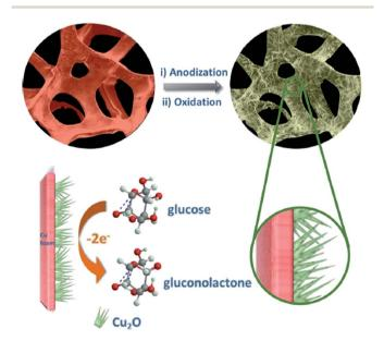
Fig. 4 Schematic illustration of the fabrication of the 3D Cu foam-supported mesoporous  $\text{Cu}_2\text{O}$  nanothorn array electrode and its function in the electrocatalytic oxidation of glucose in alkaline media. Adapted with permission from ref. 19. Copyright @ 2015 American Chemical Society.
