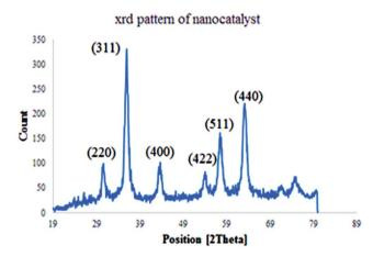
Fig. 3 The X-ray diffraction pattern of Cu(II) immobilized on Fe<sub>3</sub>-O<sub>4</sub>@SiO<sub>2</sub>@L-arginine nanoparticle.
