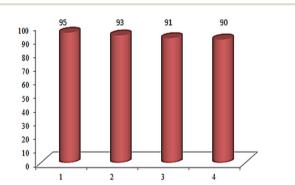
Fig. 5 Reusability of the Cu( $_{\rm II}$ ) immobilized on Fe $_3O_4$ @SiO $_2$ @L-arginine for the synthesis of 5-(4-chlorophenyl)-1H-tetrazole.
