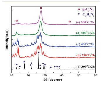
Fig. 8 XRD patterns of g- $C_3N_4$  synthesized at different temperatures for 2 h (reproduced from ref. 22, licence number 3767470249553).
