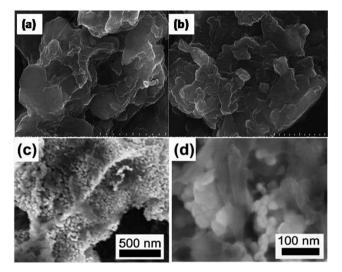
Fig. 14 SEM images of: (a)  $g-C_3N_4$ , (b)  $g-C_3N_4-FeO$  composite (c)  $g-C_3N_4-ZnO$  (8.4), and (d)  $g-C_3N_4-ZnO$  (15.6) (reproduced from ref. 80 and 85).
