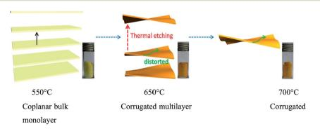
Fig. 6 Fabrication structure of distorted carbon nitride nanosheets (reproduced with permission from ref. 42, Copyright American chemical society, 2014).
