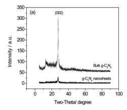
Fig. 9 XRD patterns of g-C<sub>3</sub>N<sub>4</sub> nanosheets after exfoliation (reproduced from ref. 40, licence number 3767461234354).
