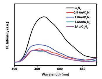
Fig. 19 PL spectra of neat  $g-C_3N_4$  and  $Au/g-C_3N_4$  nanocomposites (reproduced from ref. 70).
