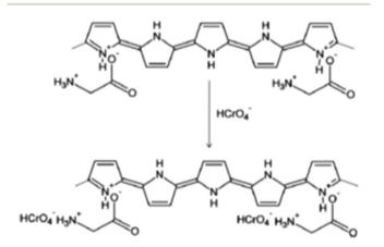
Scheme 2 The plausible adsorption mechanism for the removal of Cr(II) ions using the PPy-gly adsorbent.<sup>38</sup>
