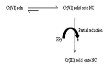
Scheme 5 The mechanism for adsorption and partial reduction of Cr(vi) onto the PPy-OMMTC nanocomposite.<sup>123</sup>
