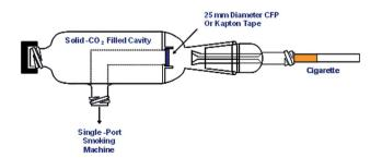
Fig. 1 A schematic of the smoking glassware with a dry ice chamber. The cigarette is fitted into the glass tube on the right and a plastic tube is used to connect to a single-port smoking machine. During the experiment, the glass tube was inserted further so that the smoke from the cigarettes sticks to the CFP or a Kapton tape directly. The cap for the dry ice chamber is not kept tight during smoking in order to prevent any increase in pressure in the chamber.
