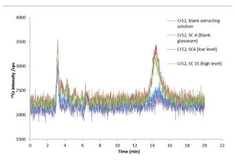
Fig. 6 HPLC-ICP-MS chromatogram of Cr species in mainstream smoke from cigarette spiked two different spike levels (5.80 and 9.80 μg g<sup>-1</sup> of chromium, respectively) using 2.8 mM TPABr and 4 mM EDTA (pH 8.5) as extractant. 0.18 mM, 1 mM EDTA (pH 8) as mobile phase at a flow rate of 0.8 mL min<sup>-1</sup>
