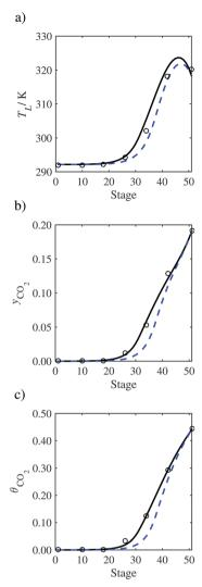
Fig. 8 Sensitivity analysis of the mass transfer correlation on the profiles predicted with our model compared with the experimental pilot-plant data of Run T22<sup>13</sup>: mass-transfer correlations from Onda et al.  $^{57.58}$  (continuous curve); mass-transfer correlations from Rocha et al.  $^{60.151}$  (a) Temperature profile for the liquid phase, (b) gas phase  $CO_2$  concentration profile, and (c) liquid phase  $CO_2$  loading. Stage 50 corresponds to the bottom of the column.
