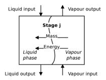
**Fig. 5** A schematic of a non-equilibrium stage. This stage represents a section of packing in a packed column.
