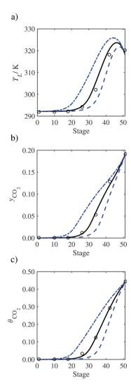
Fig. 20 Sensitivity analysis of the  $CO_2$  diffusivity in the liquid phase on the profiles predicted with our model in terms of the scaling parameter  $\tau$  compared with the experimental pilot-plant data of Run T22 of Tontiwachwuthikul et al.:  $^{13}\tau=0.041$  (continuous curve),  $\tau=0.082$  (dashed curve), and  $\tau=0.021$  (dot-dashed curve). (a) Temperature profile for the liquid phase, (b) gas-phase  $CO_2$  concentration profile, and (c) liquid-phase  $CO_2$  loading.
