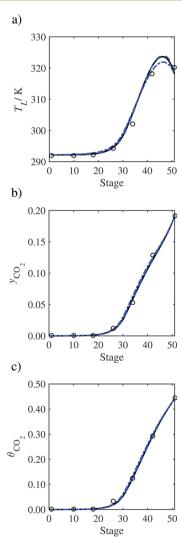
Fig. 23 Sensitivity analysis of the vapour-phase heat-transfer coefficient on the profiles predicted with our model compared with the experimental pilot-plant data of Run T22 of Tontiwachwuthikul *et al.*:  $^{13}$  Nominal value (continuous curve), coefficient value multiplied by 10 (dashed curve), and coefficient value divided by 10 (dot-dashed curve). (a) Temperature profile for the liquid phase, (b) gas-phase  $CO_2$  concentration profile, and (c) liquid-phase  $CO_2$  loading.
