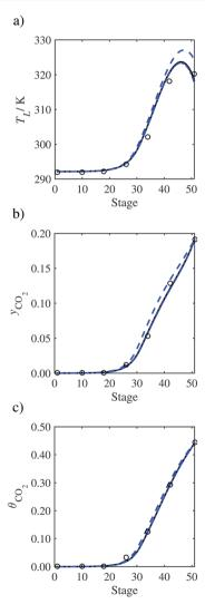
Fig. 25 Sensitivity analysis of the amount of water in the inlet flue gas on the profiles predicted with our model compared with the experimental pilot-plant data of Run T22 of Tontiwachwuthikul  $et\,al.:^{13}$  Nominal value (continuous curve),  $y_{\rm H_2O}=0.072$  (dashed curve), and  $y_{\rm H_2O}=0$  (dot-dashed curve). (a) Temperature profile for the liquid phase, (b) gas-phase  $\rm CO_2$  concentration profile, and (c) liquid-phase  $\rm CO_2$  loading.
