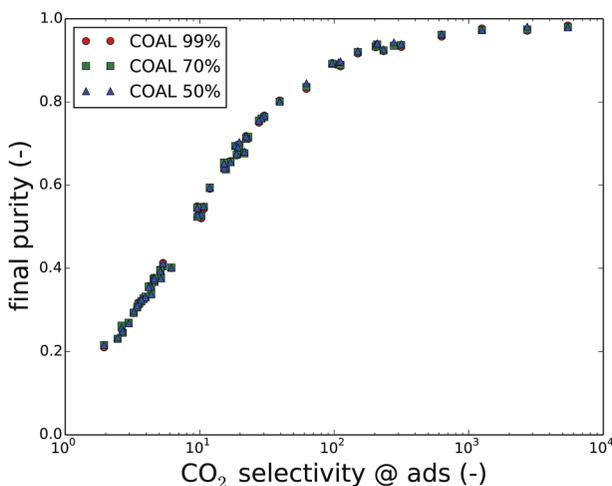
Fig. 6 The final purity as a function of the CO<sub>2</sub>/N<sub>2</sub> selectivity of the material at adsorption conditions for carbon capture from coal flue gases at different imposed purities (99%, 70%, 50%). Note that the selectivity is a material property, the imposed purity an adaptable process parameter and the final purity an outcome of the process optimization.
