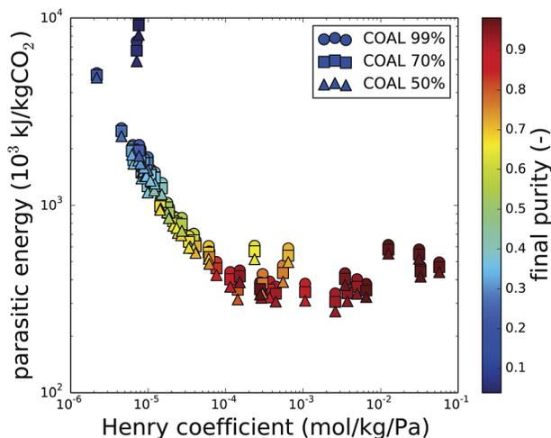
Fig. 5 The parasitic energy to capture CO<sub>2</sub> from coal flue gas as a function of the CO<sub>2</sub> Henry coefficient ( $k_{H,CO_2}$ ) at 300 K, for CO<sub>2</sub> at 99%, 70% or 50% and 1 bar. The color code indicates the purity of the final gas mixture and shows that the purity requirement of 99% is only obtained for the best performing materials.
