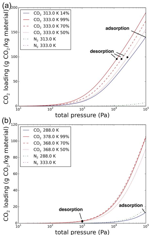
Fig. 8 The CO<sub>2</sub> and N<sub>2</sub> isotherms of NaX for carbon capture from coal-fired power plant flue gases (a) and direct air capture (b), respectively. The adsorption and different desorption conditions indicated are depending on the imposed purity of the CO<sub>2</sub>.
