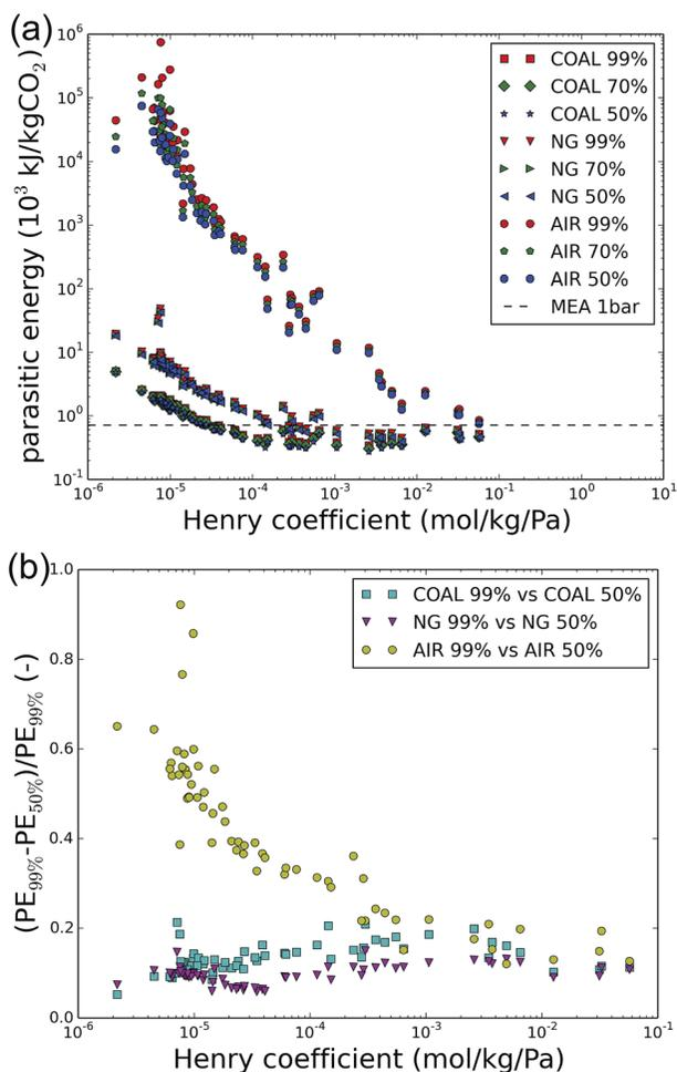
Fig. 4 (a) The parasitic energy to capture CO<sub>2</sub> from a coal-fired power plant (COAL), a natural gas-fired power plant (NG) or directly from air (AIR). Final purity requirements of 50, 70 and 99% are shown and 1 bar is maintained across all cases. (b) The relative gain in parasitic energy (PE) between the parasitic energy for 50% versus 99% imposed purity for coal flue gases, natural gas flue gases and ambient air.
