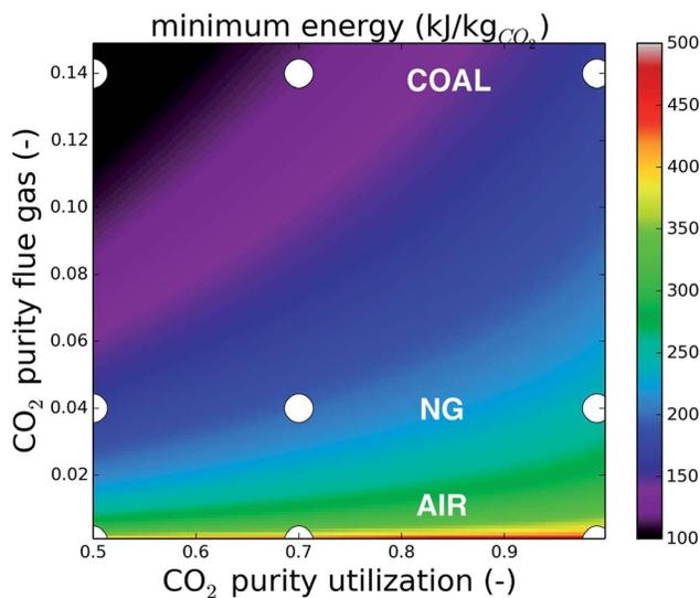
Fig. 2 The minimum energy (in  $\text{kJ kg}_{\text{CO}_2}^{-1}$ ) to separate  $\text{CO}_2$  from a binary mixture with an initial content (y-axis) to a final composition (x-axis), at 313 K and 1 bar. The points relevant in this manuscript are shown in white. The adsorption temperature in the case of direct air capture is 288 K in this manuscript, which lowers the minimum energy compared to the values in this figure.
