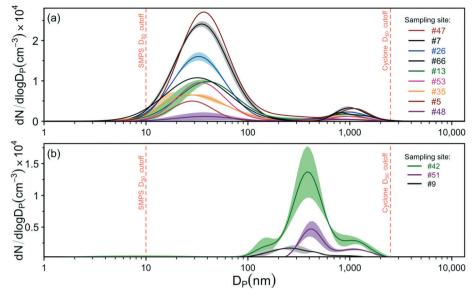
Fig. 4 Aerosol size distributions of aerosolized samples presenting a primary peak <100 nm (a) and those with a primary peak >100 nm (b). Shaded areas represent standard errors to the mean values. Curves with no shaded regions represent situations in which only one sample was aerosolized due to insufficient sample mass for replicates. The residual standard deviation (RSD) at the peak measurement in site #42 (the broadest distribution) is 30%.
