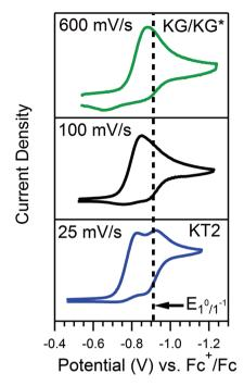
Fig. 6 CVs of a solution of 0.5 mM 1 and 0.5 mM 4-trifluoromethoxy-anilinium (p $K_a = 9.28$ ) produced at different scan rates, as denoted. All voltammograms recorded in a 250 mM [Bu<sub>4</sub>N][PF<sub>6</sub>] CH<sub>3</sub>CN solution.
