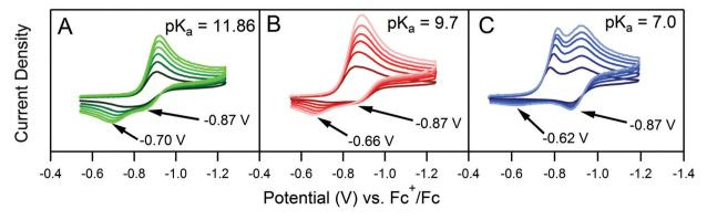
Fig. 2 Three sets of cyclic voltammograms recorded from solutions containing 0.5 mM 1 and 0.5 mM (A) 4-methoxyanilinium, (B) 4-chloroanilinium, (C) 4-cyanoanilinium. Each set of data consists of six voltammograms recorded at 100, 200, 300, 400, 500, and 600 mV s<sup>-1</sup>. All voltammograms recorded in a 250 mM [Bu<sub>4</sub>N][PF<sub>6</sub>] CH<sub>3</sub>CN solution.
