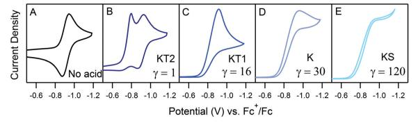
Fig. 3 Cyclic voltammograms of a 0.5 mM solution of 1 with (A) 0 mM; (B) 0.5 mM; (C) 8.0 mM; (D) 15 mM; (E) 60 mM 4-trifluoromethylanilinium. All voltammograms recorded at 100 mV s<sup>-1</sup> in 250 mM [Bu<sub>4</sub>N][PF<sub>6</sub>] CH<sub>3</sub>CN solution.
