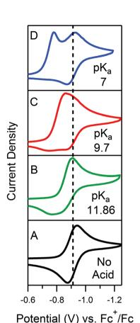
Fig. 5 CVs of 0.5 mM 1 in the presence of 0.5 mM of the respective anilinium derivative. (A) No acid; (B) 4-methoxyanilinium; (C) 4-chloro-anilinium; (D) 4-cyanoanilinium. All voltammograms recorded at 100 mV s<sup>-1</sup> in a 250 mM [ $Bu_4N$ ][ $PF_6$ ] CH<sub>3</sub>CN solution.
