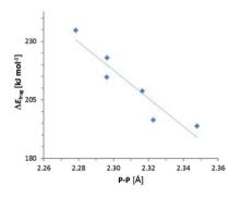
Fig. 5 Plot of computed fragmentation energies  $\Delta E_{\rm frag}$  vs. bond distances. The straight line is the result of a linear regression analysis ( $R^2$  = 0.89).
