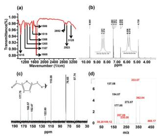
Fig. 1 (a) FT-IR, (b) <sup>1</sup>H NMR, (c) <sup>13</sup>C NMR and (d) MALDI-mass spectra of sucrose-derived CDs (S-CDs).
