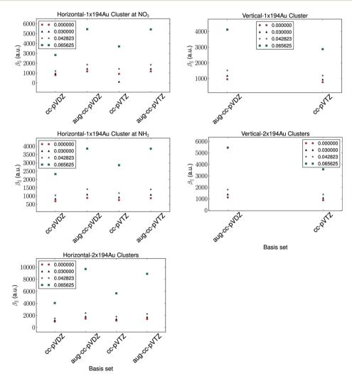
Fig. 2 The basis set dependence of the hyperpolarizability with a fixed cluster size of 194 Au atoms and a fixed vertical distance of 1.95 Å and a horizontal distance of 2.4 Å
