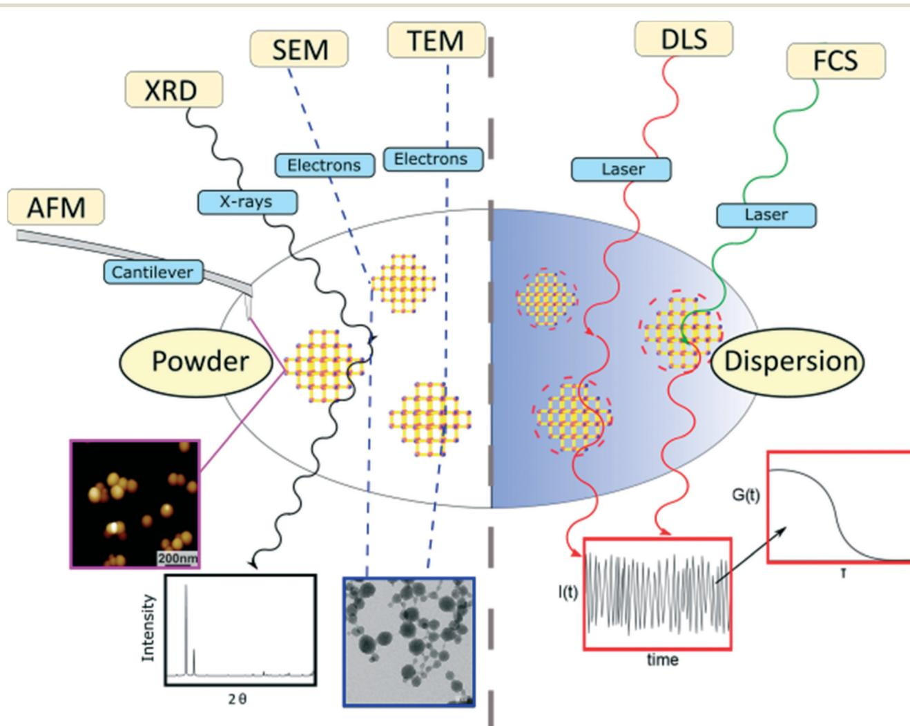
**Fig. 1** | Overview of the methods used to determine the size of Zr-fum MOF nanoparticles (atomic-force microscopy (AFM), X-Ray diffraction (XRD), transmission electron microscopy (TEM), scanning electron microscopy (SEM), dynamic light scattering (DLS) and fluorescence correlation spectroscopy (FCS)).
