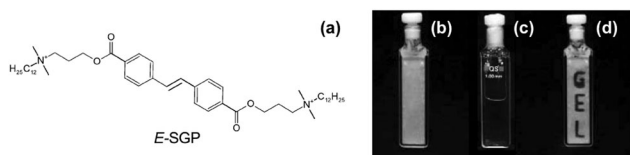
Fig. 8 Molecular structure of alkene-based photoresponsive LMWG. On exposure to UV light, a trans -to- cis isomerisation occurs, leading to a gel-to-sol transition. Reproduced from ref. 39 with permission of the Royal Society of Chemistry.
