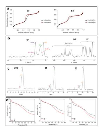
Fig. 1 (a) Nitrogen adsorption-desorption isotherms of materials S3 and S4. (b) 13C-CP MAS NMR spectra of materials S1 and S2. (c) 29Si MAS NMR spectra of materials KIT-6, S1 and S2. (d) Thermogravimetric analysis of materials \$1-\$6.
