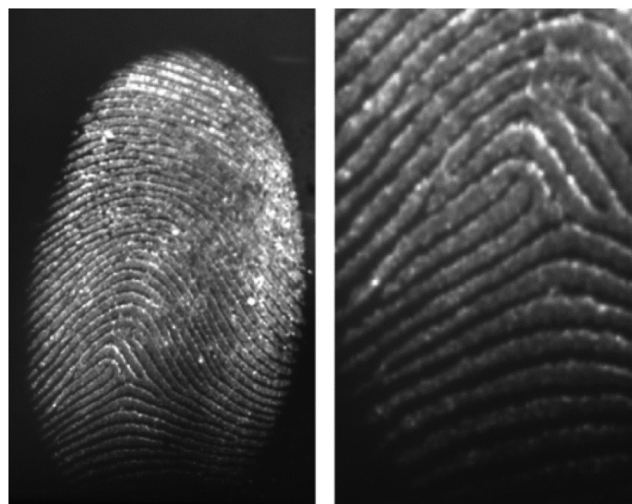
Fig. 11 A charged latent fingerprint on a PVDF substrate developed by using the aptamer-based reagent. The fingerprint was aged for 24 hours before it was developed with the lysozyme aptamer 1 reagent containing CAL Fluor® Orange 560 as the fluorescent tag. 91 Reproduced from ref. 91 with permission from Wiley.
