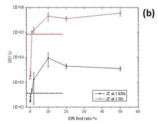
Fig. 7 (a) Impedance amplitude of PEDOT and PEDOT-co-EPh copolymers as a function of frequency; (b) impedance amplitude at 1 Hz and 1 kHz for the PEDOT-co-EPh copolymers as a function of EPh content; dashed lines indicate the impedance amplitude of bare Pt electrode at 1 Hz (red) and 1 kHz (black), respectively (deposition charge: 288 mC cm $^{-2}$ ).
