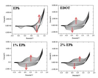
Fig. 2 First 10 cycles of CV recorded during potentiodynamic polymerizations in monomer solutions (versus Ag/AgCl). Red arrows indicate expanded CV curves after each cycle
