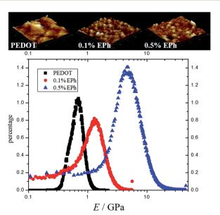
Fig. 8 AFM QNM modulus distribution. (a) AFM image of the polymer films (2  $\mu m$  by 2  $\mu m$ ); (b) AFM QNM modulus distribution of PEDOT, 0.1% EPh and 0.5% EPh.
