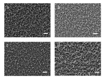
Fig. 8 SEM images of (a) P(ProDOT-diene); (b) EH-thiol modified PProDOTdiene; (c) PEO-thiol modified P(ProDOT-diene); (d) ferrocene-thiol modified PProDOT-diene (scale bar represents 2 μm).
