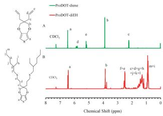
Fig. 1 Chemical structure and  $^1\mathrm{H}$  NMR spectra in CDCl $_3$  of (A) ProDOT-diene and (B) ProDOT-diEH.
