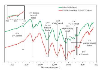
**Fig. 6** FTIR spectra of P(ProDOT-diene) and EH-thiol modified P(ProDOT-diene). Part of the characteristic absorption bands are labelled with wavenumbers.
