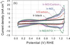
Fig. 6 Electrocatalytic performance of Ir-ND catalysts in a single PEM electrolyzer cells: (a) Membrane Electrode Assembly (MEA) polarization curves with a catalyst loading of 1.0 mg cm $^{-2}$  and (b) cyclic voltammograms, 50 mV s $^{-1}$ . Other conditions: 80 °C cell temperature, 5 cm $^{2}$  active electrode area, preheated 80 C deionized water was supplied at 1.5 mL min<sup>-1</sup>.
