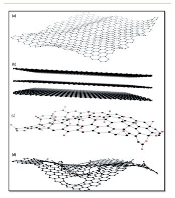
**Fig. 4** Representative chemical structures of some of the members of GFNs: (a) graphene, (b) few-layer graphene, (c) graphene oxide (oxygen atoms are in red), and (d) reduced graphene oxide.<sup>167</sup>
