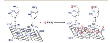
Fig. 7 EDTA-modified GO and its interaction with bivalent heavy metal ions.<sup>75</sup>
