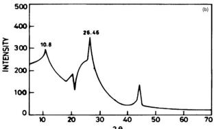
Fig. 5 (a) Typical Raman spectra $^{23}$  and (b) XRD patterns $^{25}$  of graphene.
