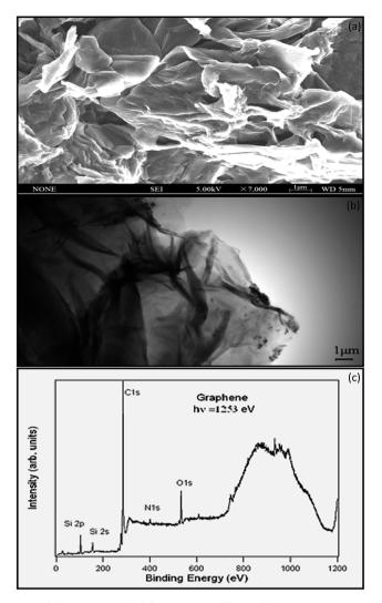
Fig. 6 (a) SEM image, $^{85}$  (b) TEM image, $^{85}$  and (c) wide XPS scan of cleaved UITAR $^{25}$  of graphene.
