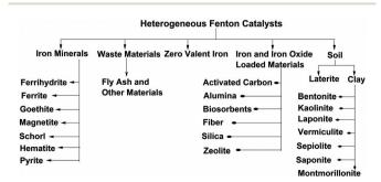
Fig. 2 Classification of heterogeneous Fenton catalysts.
