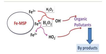
Fig. 5 Contaminant degradation mechanism of Fe-MSP. Figure taken from ref. 150.
