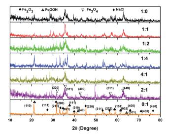
Fig. 3 XRD spectra of magnetite prepared with various ferrous-toferric ion ratios. Taken from Ref. 80.
