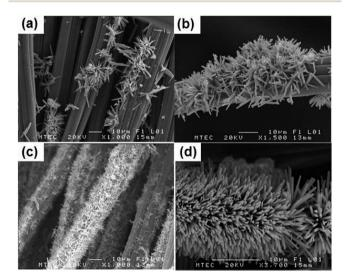
Fig. 16 SEM images of the as-grown ZnO NRs on ACC using a hydrothermal method: growth time (a) 10 hours (no pre-treatment of ACC or pH control during growth); (b) 10 hours and (c) 15 hours (the hydrothermal process was conducted with pre-treatment of the seeded ACC substrates by dipping then into a 20 mM precursor solution); (d) 10 hours (using the hydrothermal method by adjusting the pH to 6.8 to 6.9 at the initial state). (Reproduced with permission from ref. 115.)
