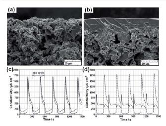
Fig. 27 SEM images of (a) uncoated carbon electrodes and (b) carbon electrodes coated with an ion-exchange polymer; the conductivity transient of effluent measured at a cell potential of (c) 1.2 V with a flow rate of 20 mL min $^{-1}$  and (d) -1.5 V with a flow rate of 20 mL min $^{-1}$ . Solid line: MCDI cell, dashed line: CDI cell. (Reproduced with permission from ref. 140.)
