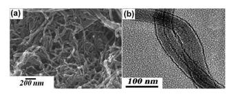
**Fig. 2** SEM and TEM images of CNTs. (Reproduced with permission from ref. 59.)
