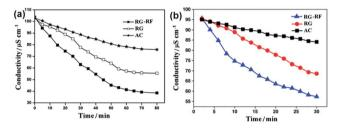
Fig. 25 Comparative results of RGO-RF, RGO and AC electrodes in terms of electrosorption performance in (a) 40 mg L<sup>-1</sup> FeCl<sub>3</sub> solution and (b) 40 mg L<sup>-1</sup> NaCl solution. (Reproduced with permission from ref. 129 and 130.)
