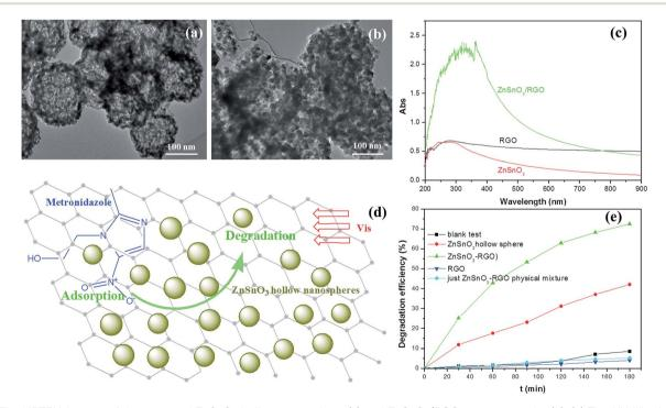
Fig. 3 The HRTEM images of the prepared ZnSnO<sub>3</sub> hollow nanosphere (a) and ZnSnO<sub>3</sub>/RGO nanocomposite (b). (c) The UV-Vis absorption spectra of the RGO, pure  $ZnSnO_3$  hollow nanosphere and  $ZnSnO_3/RGO$  nanocomposite. The speculated illustration (d) and degradation efficiencies (e) of the metronidazole wastewater by ZnSnO3 hollow nanosphere and ZnSnO3/RGO nanocomposite photocatalysts under visible light irradiation. Reproduced with permission from ref. 33.
