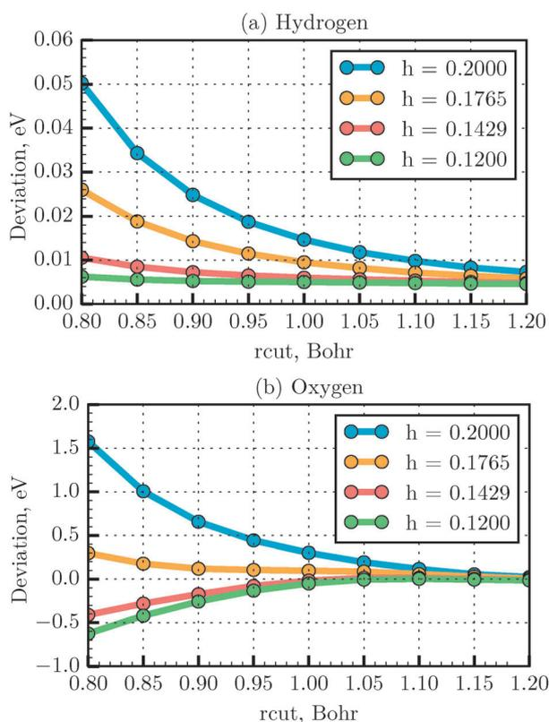
Fig. 5 Convergence of total energy with respect to all-electron energy using TFD1W theory for various rcut values and different grid spacings, calculated for the H (a) and O (b) atoms, respectively.
