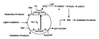
Fig. 2 Pictorial representation of indirect dye degradation process.<sup>24</sup>
