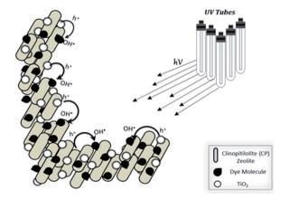
Fig. 8 Synergistic effect of  ${\rm TiO_2}$  and clinopitilolite catalyst on dye degradation by producing OH free radicals. <sup>318</sup>
