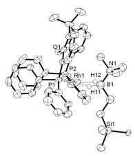
Fig. 1 Solid-state structure of the cationic portion of 3. Displacement ellipsoids are drawn at the 50% probability level. [BArF4] anion and all carbon-bound H atoms are omitted for clarity. Only the major component of the disordered NMe<sub>3</sub> and SiMe<sub>3</sub> groups are shown. Selected bond lengths (Å) and angles (°): Rh1-P1, 2.2398(18); Rh1-P2, 2.2670(17); Rh1-O1, 3.2342(73); Rh1-B1, 2.179(7); B1-N1, 1.603(4); P1-Rh1-P2, 98.23(6).
