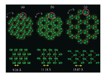
Fig. 10 Simulated crystal structures of the MIL-88A framework in its  $\bf np$  (a),  $\bf as$  (b), and  $\bf lp$  (c) forms. (Reprinted with permission. <sup>87</sup> Copyright 2005 American Chemical Society.)
