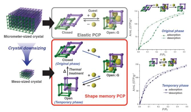
Fig. 7 Schematic depiction of the flexible behaviour of micro-sized  $[Cu_2(bdc)_2(bipy)]_n$  in comparison with meso-sized  $[Cu_2(bdc)_2(bipy)]_n$ . Right – methanol adsorption isotherms of the closed (original phase) and the open (temporary phase) of meso-sized [Cu<sub>2</sub>(bdc)<sub>2</sub>(bipy)]<sub>n</sub>. (Reprinted with permission.<sup>76</sup> Copyright 2013. American Association for the Advancement of Science.)
