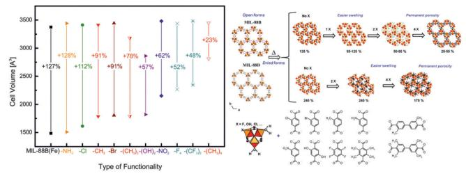
Fig. 18 Left: depiction of the evolution of the cell volumes during the swelling process depending on the functionalities added at the bdc benzene core of MIL-88B(Fe) Right: schematic depiction of the pore swelling in MIL-88B and MIL-88D depending on the number of substituents on the benzene rings. (Reprinted with permission.<sup>140</sup> Copyright 2011. American Chemical Society.)
