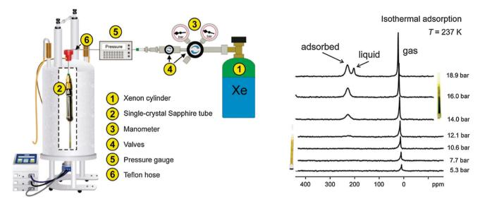
Schematic representation of an apparatus for high pressure in situ 129Xe NMR experiments under variable thermodynamic conditions (left). In situ 129Xe NMR spectra recorded during the adsorption and desorption of Xenon on DUT-8(Ni) at 237 K (right). (Reprinted with permission 180 Copyright 2011. American Chemical Society.)
