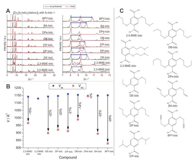
Fig. 17 (A) Powder patterns of as-synthesized (black) and dried (red)  $[Zn_2(fu-bdc)_2(dabco)]_n$ . (B) Evolution of the cell paramters during the transitions from the as-synthesized lp to the dried np of the framework. (C) Listing of the linkers that were used to prepare the discussed pillared-layered frameworks. (Reprinted with permission.<sup>138</sup> Copyright 2012. American Chemical Society.)
