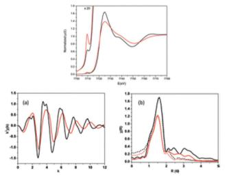
Fig. 28 Top: cobalt K-edge XANES spectra of 1 (black) and 1' (red) pre edge feature at 7709.5 eV shown with 20× magnification. Bottom: comparison between EXAFS spectra of 1 and 1' in (a) k space and (b) FT R space (also includes the theoretical first shell fits); see text for details of fitting. (Reprinted with permission.<sup>190</sup> Copyright 2012 American Chemical Society.)
