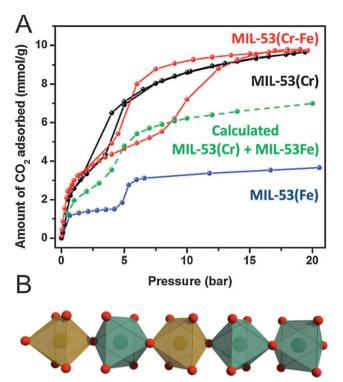
Fig. 20 (A) Comparison of the CO<sub>2</sub> adsorption isotherms of MIL-53(Fe-Cr), MIL-53(Fe), and MIL-53(Cr). (B) One dimensional SBU chains in MIL-53(Fe-Cr). Green and orange polyhedra represent iron and chromium SBUs, respectively. Red spheres represent oxygen atoms. (Reprinted with permission.<sup>151</sup> Copyright 2012. The Royal Society of Chemistry.)
