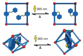
Fig. 4 Illustration of the photochemically induced phase transitions in metal-organic frameworks. Top: Linker functionalization with photoswitchable units in a rigid MOF. Bottom: employment of a photoswitch in a host-quest fashion into a flexible MOF.
