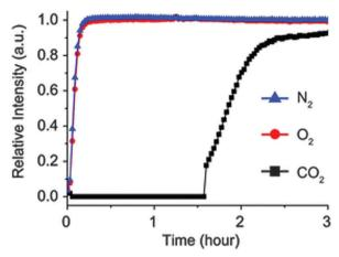
Fig. 31 Breakthrough curve for CID-3 for mixture  $CO_2: O_2: N_2 = 1: 21: 78$ at total pressure of 0.5 MPa. (Reproduced with permission.  $^{22\overline{3}}$  The Royal Society of Chemistry.)
