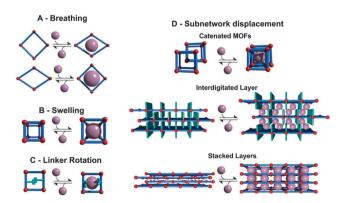
Fig. 2 Classification of different flexibility modes of MOFs. One class is characterized by the change in unit cell volume ( $\Delta V \neq 0$ ; A, B and D) while in the other case the unit cell volume does not change ( $\Delta V = 0$ ; C, D).
