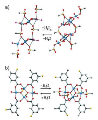
Fig. 23 Structural transformations in Cu-SIP-3 during hydration/ dehydration: (a) Chains of the copper tetramers in the low-temperature (left) and high-temperature (right) structures. (b) Copper tetramers in the low-temperature (left) and high-temperature (right) structures. Color codes: Blue balls - copper atoms; red balls - oxygen atoms; yellow balls sulfur atoms; grey balls – carbon atoms (Reprinted with permission from. 155 Copyright 2010. American Chemical Society.)
