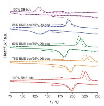
Fig. 21 DSC curves of  $[Zn_2(BME-bdc)_{2x}(DB-bdc)_{2-2x}dabco]_n$  solid solutions. (Reprinted with permission.<sup>57</sup> Copyright 2013 John Wiley and Sons) and Sons.
