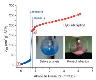
Fig. 33 Color change of [Co<sub>1.5</sub>(tipb)(SO<sub>4</sub>)(bdc)<sub>0.5</sub>]<sub>n</sub> during H<sub>2</sub>O adsorption. (Reprinted with permission. 228 Copyright 2012 John Wiley and Sons.)
