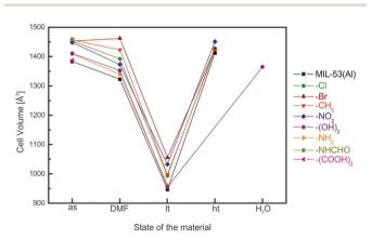
**Fig. 16** Evolution of the cell volume in MIL-53(Al) materials depending on the treatment of the material.
