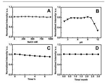
**Fig. 4** (A) The relative fluorescence intensity at 427 nm (excitation at 344 nm) of the FNCPs in the NaCl solution. (B) Dependence of the fluorescence intensity on the pH values from 2 to 12. (C) The variation of the fluorescence intensity of the FNCPs under irradiation by a 500 W Xe lamp for different time intervals. (D) Photostability of the FNCPs as a function of the storage time.
