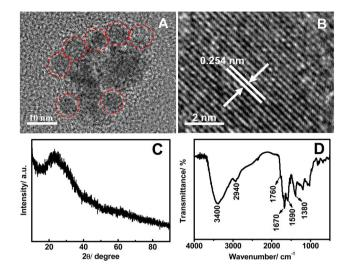
Fig. 2 Typical TEM image (A), HRTEM image (B), XRD pattern (C), and FTIR spectra (D) of the FNCPs.
