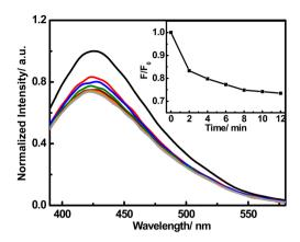
**Fig. 5** Time-dependent fluorescence responses of the FNCPs to 50  $\mu$ M Hg<sup>2+</sup>. Inset shows the  $F/F_0$  plotted against time in the presence of 50  $\mu$ M Hg<sup>2+</sup>, where F and  $F_0$  are the fluorescence intensity of the FNCPs at 427 nm with and without Hg<sup>2+</sup>, respectively.
