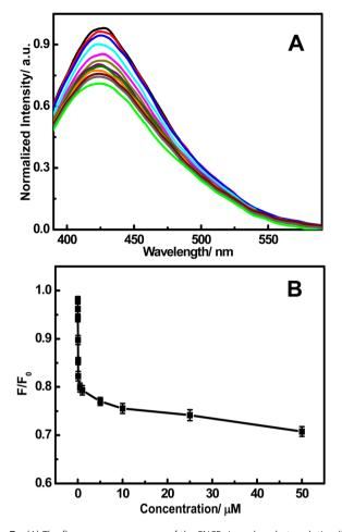
**Fig. 7** (A) The fluorescence responses of the FNCPs in a phosphate solution (25 mM, pH 7.4) after the addition of different concentrations of  $Hg^{2+}$  (top to bottom): 0, 0.010, 0.025, 0.050, 0.075, 0.100, 0.500, 1.00, 5.00, 10.0, 25.0, and 50.0  $\mu$ M. (B) Plot of the  $F/F_0$  with the concentration of  $Hg^{2+}$ .
