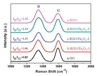
Fig. 5 Raman spectra for GO, RGO and RGO-Fe<sub>3</sub>O<sub>4</sub> composites.
