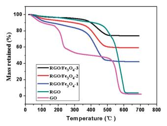
Fig. 6 TG curves of GO, RGO and RGO-Fe<sub>3</sub>O<sub>4</sub> composites in air atmosphere.
