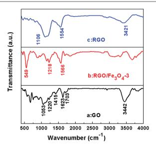
Fig. 4 FT-IR spectra of GO (a), the RGO-Fe<sub>3</sub>O<sub>4</sub>-3 composite (b) and RGO (c).
