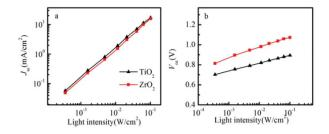
Fig. 4 The light intensity dependence of  $J_{sc}$  (a) and  $V_{oc}$  (b) in spiro-OMeTAD/ CH<sub>3</sub>NH<sub>3</sub>Pbl<sub>3</sub>/ZrO<sub>2</sub> (or TiO<sub>2</sub>) solar cells.
