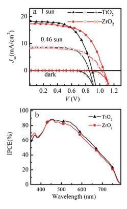
**Fig. 3** *J–V* curve in the dark and under AM 1.5G illumination of 1000 W m<sup>-2</sup> and 460 W m<sup>-2</sup> intensity. IPCE spectra of spiro-OMeTAD/CH<sub>3</sub>NH<sub>3</sub>Pbl<sub>3</sub>/ZrO<sub>2</sub> and spiro-OMeTAD/CH<sub>3</sub>NH<sub>3</sub>Pbl<sub>3</sub>/TiO<sub>2</sub> solar cell.
