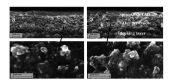
**Fig. 1** SEM image of spiro-OMeTAD/perovskite + TiO<sub>2</sub>/blocking layer/FTO using different method a: one-step deposition, b: TSD method.
