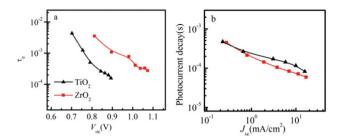
**Fig. 5** (a) Electron lifetime as a function of open circuit voltage in spiro-OMeTAD/ CH<sub>3</sub>NH<sub>3</sub>Pbl<sub>3</sub>/ZrO<sub>2</sub> (or TiO<sub>2</sub>) solar cells. (b) Photocurrent transient decay as a function of short-circuit current in spiro-OMeTAD/CH<sub>3</sub>NH<sub>3</sub>Pbl<sub>3</sub>/ZrO<sub>2</sub> (or TiO<sub>2</sub>) solar cells.
