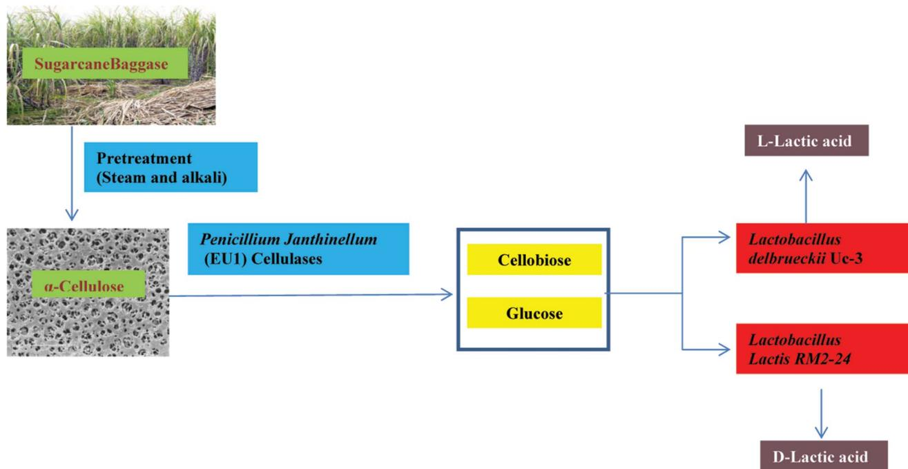
**Fig. 2** Biomass utilization through improved strains for lactic acid production using the SSAF approach. Sugarcane baggase derived cellulose is used as a substrate for lactic acid production. The cellulose is further hydrolyzed to simple sugars using cellulase produced by *P. janthinellum* (EU1). These sugars are diverted to produce D- and L-lactic acid by *L. lactis* RM2-24 and *L. delbrueckii* Uc3 using the SSAF process.
