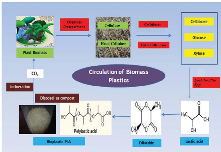
**Fig. 1** Schematic representation of the carbon cycle of bioplastics. The lignocellulosic substrate, bagasse is pretreated to remove lignin and further hydrolyzed to monomeric sugars using enzymes. These sugars are further diverted to produce lactic acid using *Lactobacillus* sp. The produced lactic acid is used as the starting material for PLA synthesis which is a biodegradable plastic. Thus, after incineration, the released carbon can be recycled in the environment.
